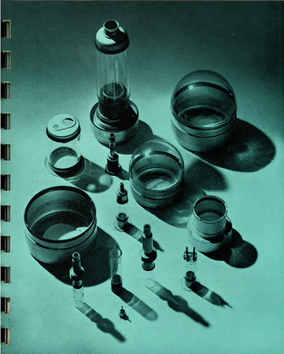
Glass-to-metal seals used in valve manufacture. The dome in the top right-hand corner is sealed to copper
