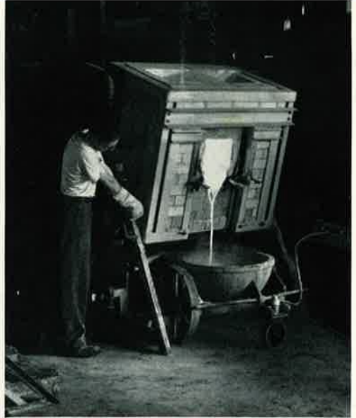
A tilting furnace at Chesterfield with platinum-lined walls to withstand corrosive action of special glasses. The tilting action permits draining and obviates the need for scraping which might damage the walls
